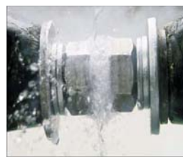
\text{O}_2 = paramagnetic (liquid here, <90\text{K} ) Clings between poles of a strong magnet
